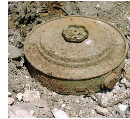
Steel-cased mines like this Russian TM-46 are vulnerable to rust in wet conditions.
