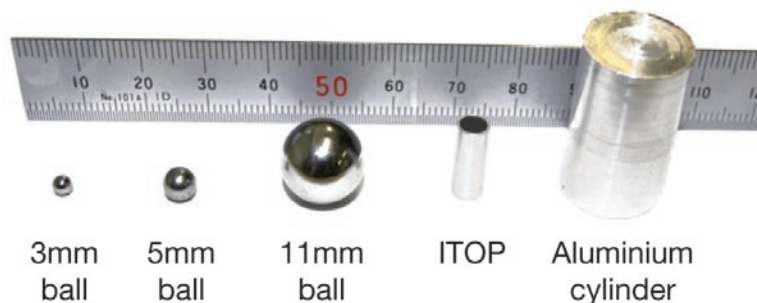
Figure 3: Metallic targets used for the discrimination experiments.
