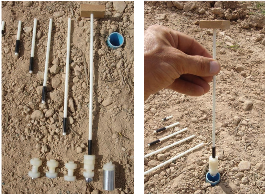
Target and target-depth set-up and insertion into the soil.
