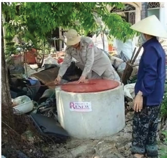
Scrap yard safe-holding container for suspected ERW. Developed by Golden West and implemented by The Vietnam Veterans Memorial Fund's Project RENEW, these containers are secured to prevent access by children. Containers are regularly checked by RENEW EOD teams.
