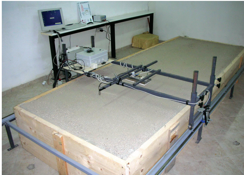
The indoor sandbox of HDL, measuring 1.3 x 3.5 x 0.5m 3 , with the active thermal detector prototype.
