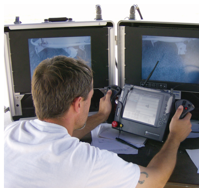
Whether operated manually or remotely, independent visual monitoring of the comb workspace is an integral part of field operation.
