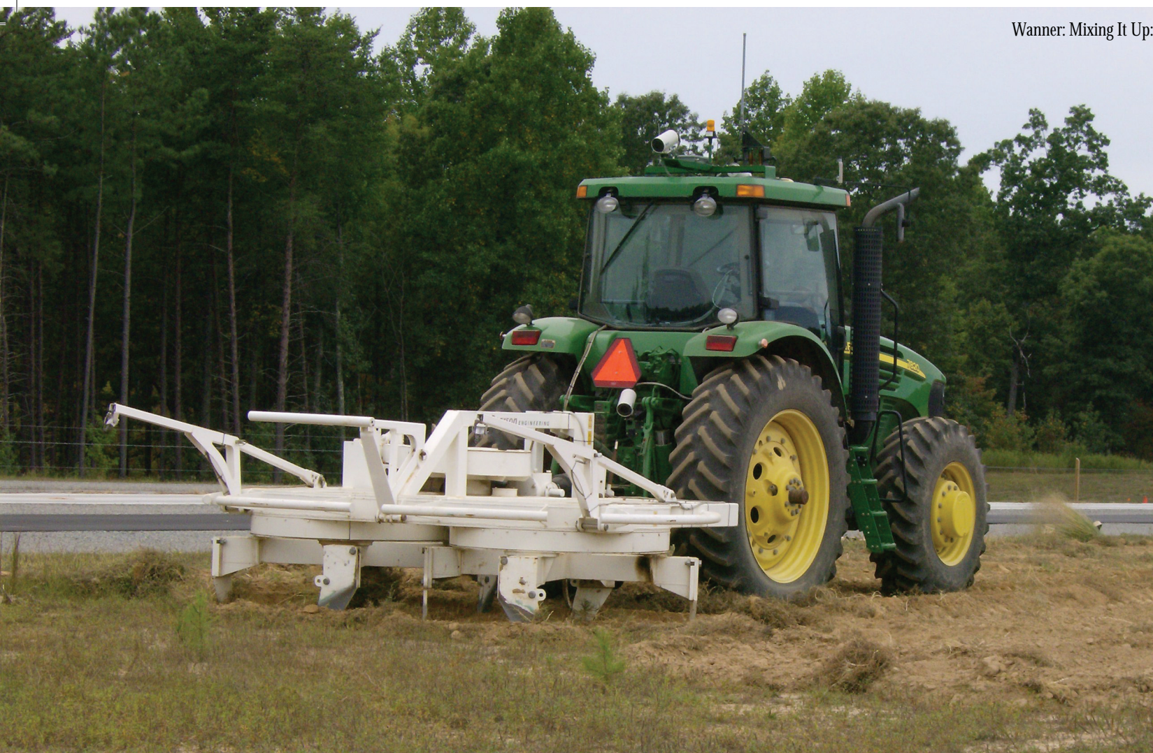
The Rotary Mine Comb combing the test minefield. ALL IMAGES COURTESY OF THE AUTHOR
