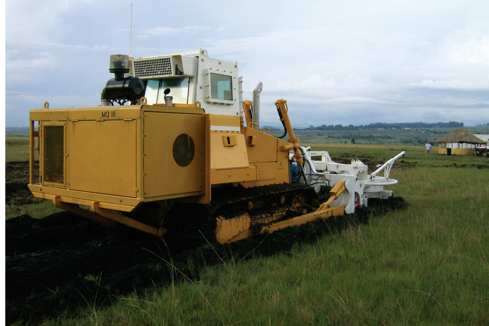
Construction dozer-mounted RMC.
