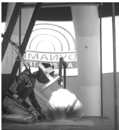
Positioning of Hybrid III anthropomorphic dummy prior to blast test on new PPE produced by ROFI. PHOTO COURTESY OF A. BREDELIUS, SWEDEC
