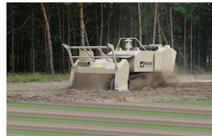
CWA 15044 performance test of the Mini MineWolf with tiller. PHOTO COURTESY OF C. BARTLING, GERMAN TEST CENTER FOR WEAPONS AND MUNITIONS
