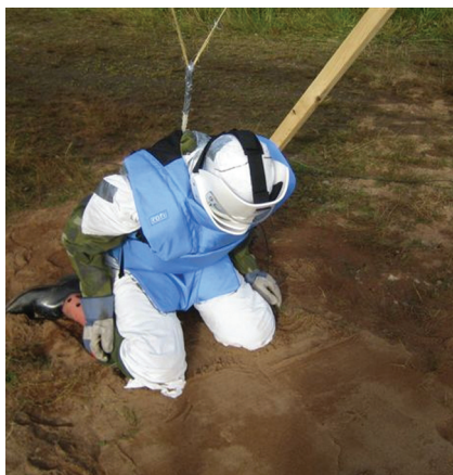
Blast test on heat-treated scratched visor. PHOTO COURTESY OF G. COLEY, DRDC-SUFFIELD
