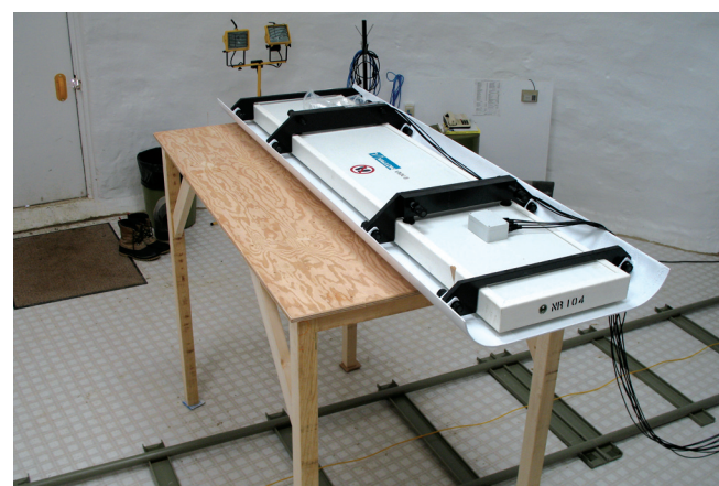
Laboratory testing of the Vallon VMV-8 metal detector array. PHOTO COURTESY OF K. RUSSELL, DRDC-SUFFIELD
