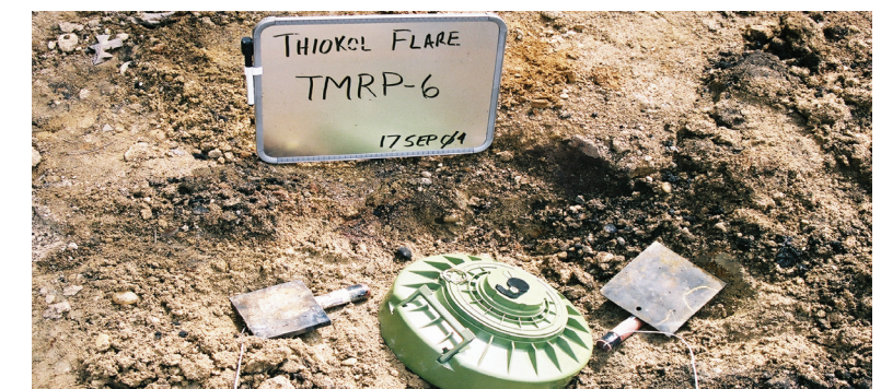
Figure 3: TMRP-6, a plastic-case AT mine with two TDFs on ground attacking mine from opposite sides with a metal plate on TDFs at ends.
