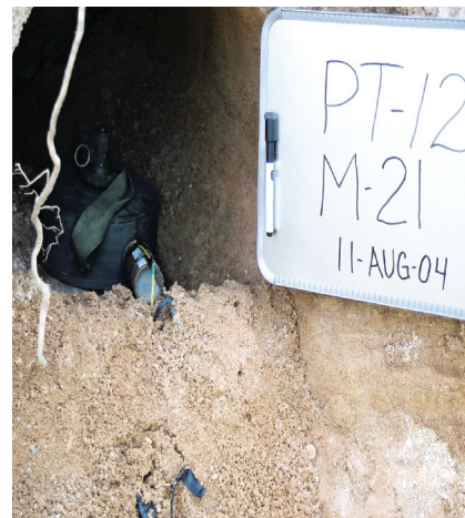
Figure 8: AT metal-case shaped-charge mine with PT-12 on a stand.
