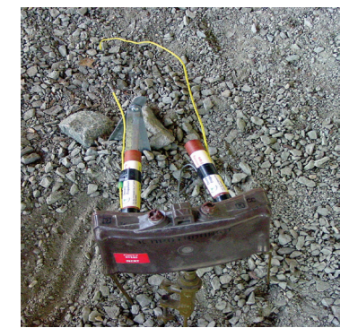
Figure 2: MON-50, AP plastic case directional mine with two TDFs attached to a stand.
