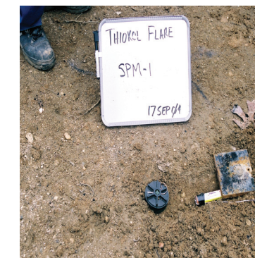
Figure 1: SPM-1, AP Thermoplastic case mine with TDF. ALL PHOTOS COURTESY OF HD R&D
