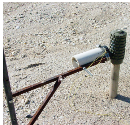
Figure 6: PMR-2A, AP stake mine with PT-12 torch on a stand.
