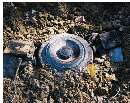
Figure 5: PT Mi-Ba-III, Bakelite-case AT mine with two PT-1s that is partially covered by the soil.
