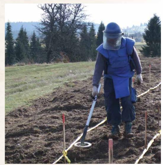
A deminer uses a metal detector in preparation for Technical Survey.
