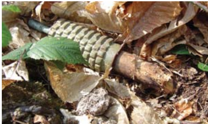
A stake mine is less likely to be initiated once the wood has rotted and the body is resting on the surface. However, once the mine becomes fixed in the ground, it may become more dangerous.
