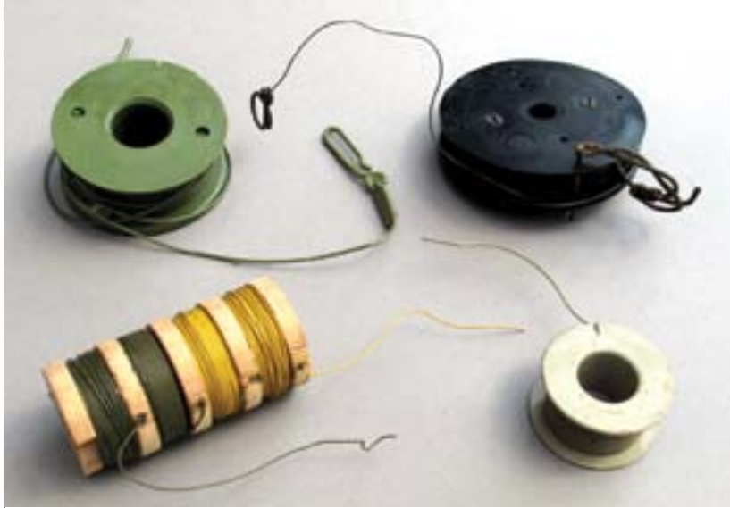
Examples of various types of tripwire. From the top left, clockwise: Former-Yugoslav, plastic-coated multi-strand stainless steel; British high-tensile steel; Italian painted soft iron; American painted soft iron.
