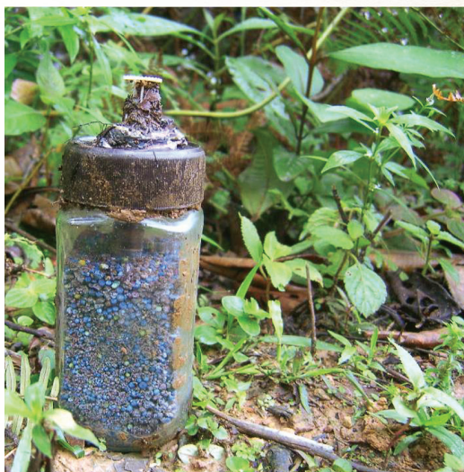
Improvised landmine, pressure activated.
