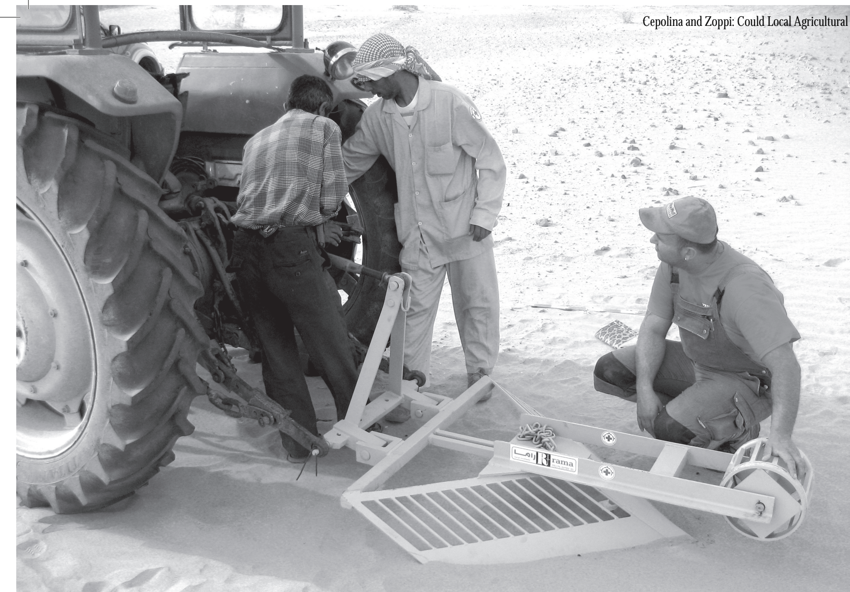
Above and opposite page: Test of the ground-processing tool designed by Snail Aid and the University of Genova in Jordan. The tractor unit here is a tractor hired locally and driven backwards.
