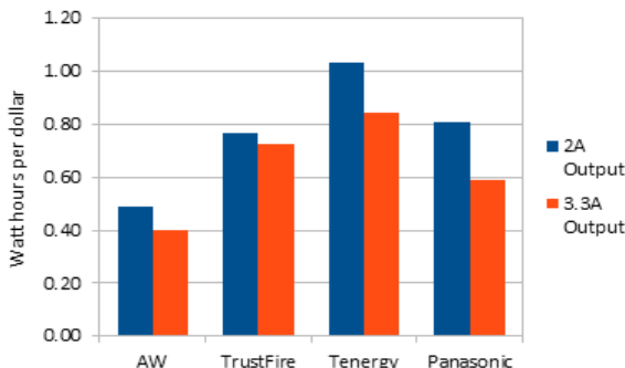
Fig. 5.1. 3: Energy density of batteries vs. cost
