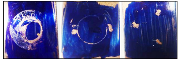
Fig. 4.2. 5: Washer contact footprints: (from left) Belleville washer, curved washer, wave washer
