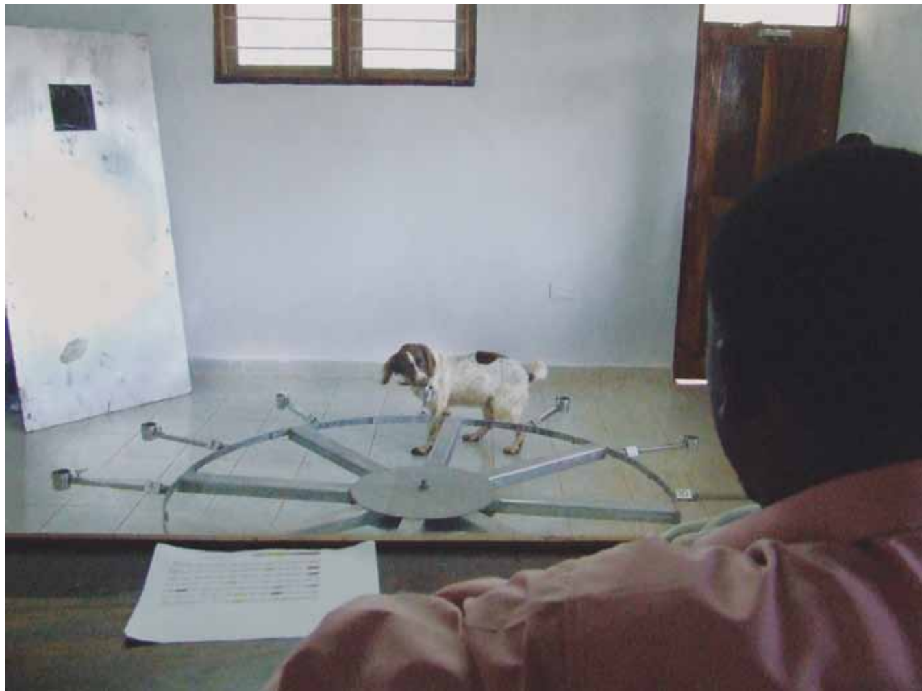
A dog sniffs a container with soil samples, some of which contain a small amount of TNT (positive sample) and others that are TNT-free (negative sample). The dog moves around the carousel, sniffing samples at the end of the arms and identifying positive samples by sitting beside them. Photo courtesy of Max Jones.
