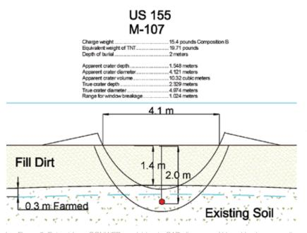
Figure 2. Extract from CONWEP overlaid onto CAD diagrams of Vung Ha clearance site showing requirements for a detonation breaking the surface of the topsoil following filling for development.
