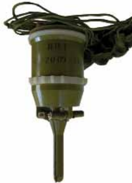
The Chinese Type 84 is a scatterable AT mine initiated by a magnetic influence fuze.
