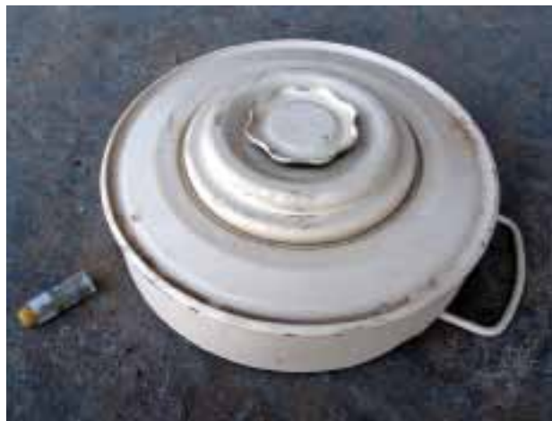
The Chinese Type 72 SP AT mine, with blast-resistant fuze to the left.
