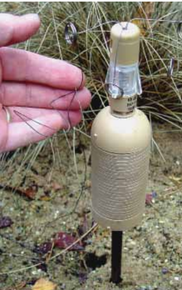
The Belgian NR 413 fragmentation mine can be initiated by any of four tripwires.
