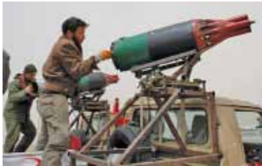
57mm air-to-ground aircraft rocket pod prepared in a ground-to-ground role mounted on a vehicle with improvised launch platform.
