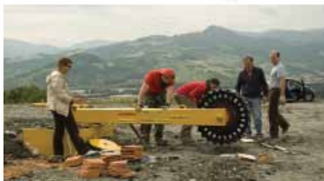
Figure 2. Pendulum digital mock-up and prototype set-up before the test.
