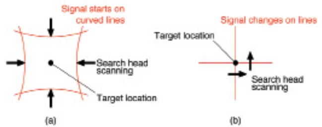
Figure 5. Pinpointing a target with (a) single-receive-coil detectors and (b) double-D coil detectors (reproduced from the STEM D Lab Test report and Metal Detector Handbook). 2,3
