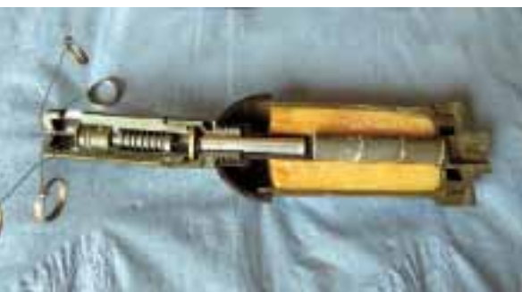
Sectioning a live NR 413 AP mine for examination.
