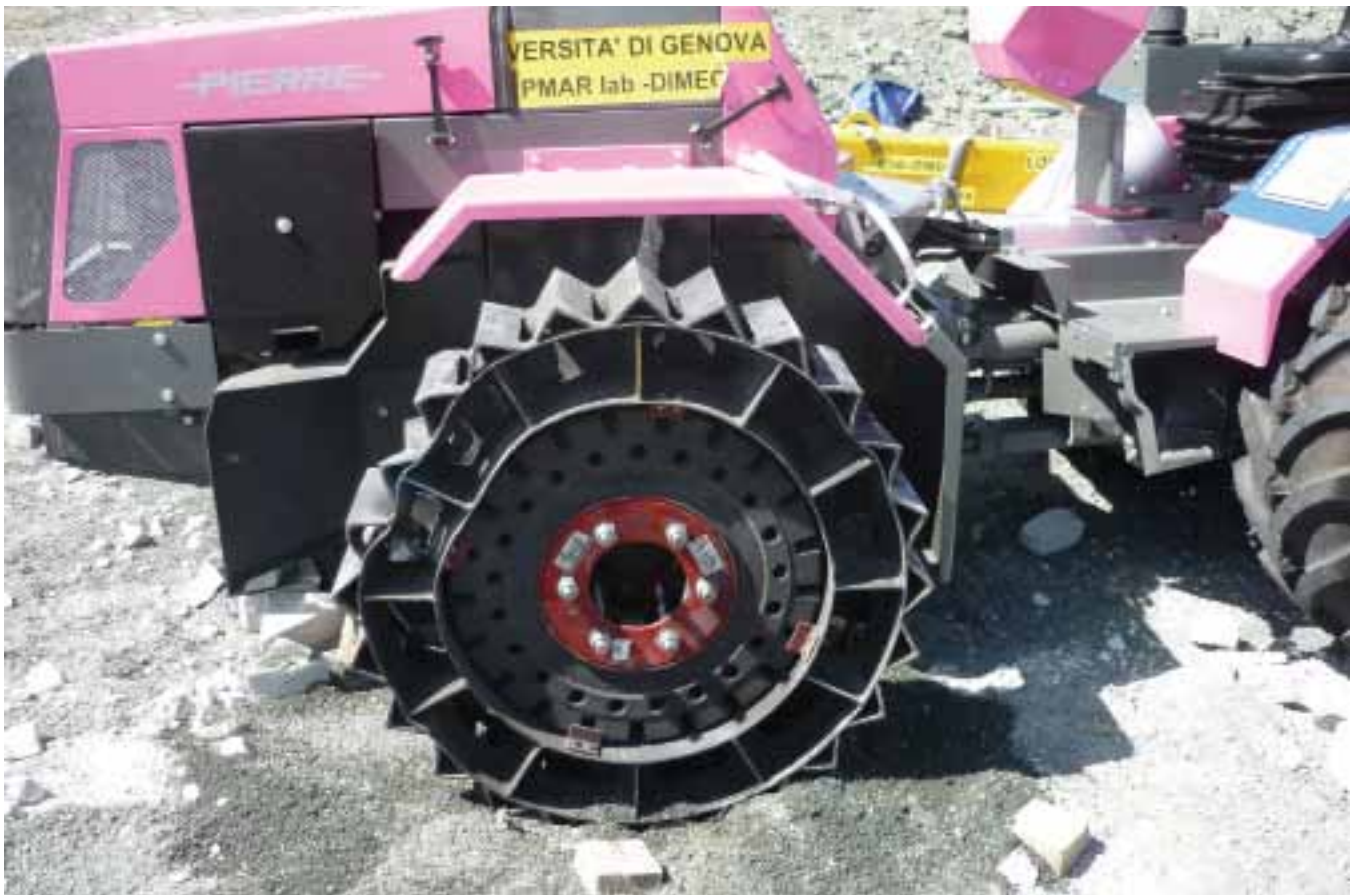
Figure 11. Genoa wheel after the fourth explosion. Only this last test was done on the tractor.
