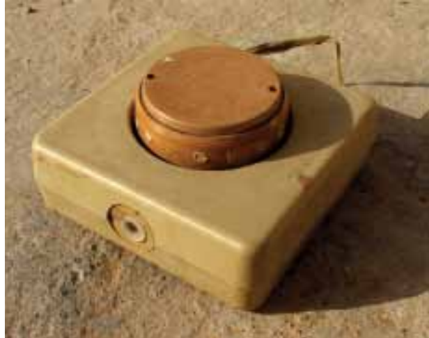
The M3A1 is a variant of the M3 which incorporates two auxiliary fuze wells.
