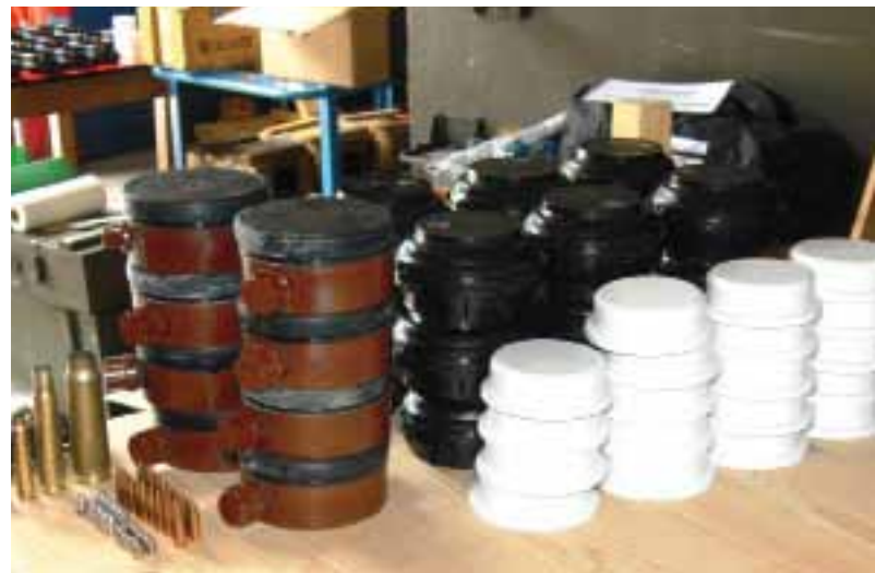
Objects used in the test. From left to right: metal clutter (ammunition belts, cartridges, bullets) and mine-like targets (Gyata-64, PPM-2, ERA calibration target).
