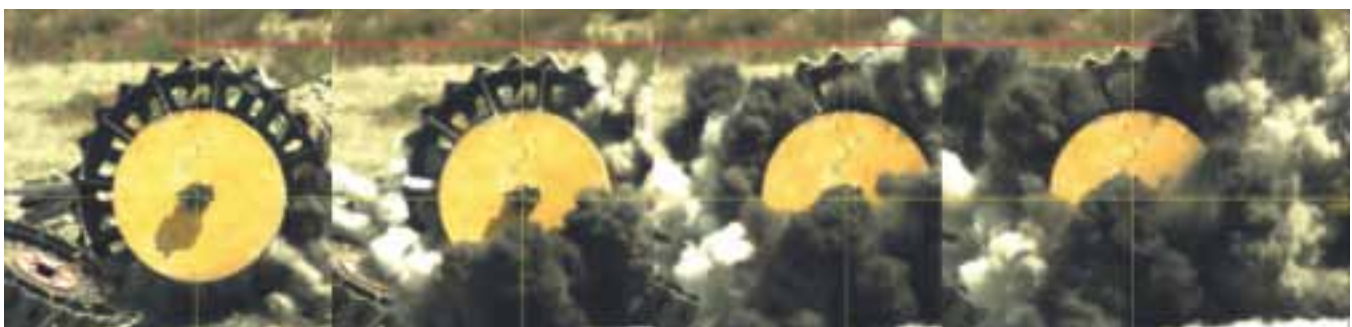
Figure 12. Frames taken by the high speed camera during the explosion of 120g of TNT under Florida wheel. The upper part of the wheel moved 73mm upwards in 1/50s while the axis did not move.
