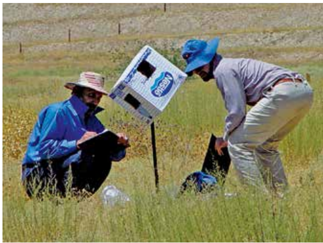
Image 2. Datum recorders with portable weather station (the temperature gauge is shaded by the box).
