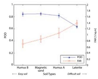
Figure 6. Performance of metal detectors in terms of POD (blue dots with solid line) and FAR (red circles and dashed line) averaged over all models tested. Soil on the left side is considered to be easy and soil on the right side is considered to be difficult. The error bars show 95% confidence bounds.
