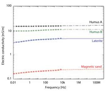
Figure 3. Frequency dependence of electric conductivity of the test soils. The dots and lines show the measured values and model fits, respectively.
