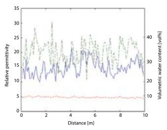
Figure 5. Spatial distribution of relative permittivity of the test soils measured in 10-m long profiles and corresponding water content determined by an empirical equation.<sup>11</sup>
