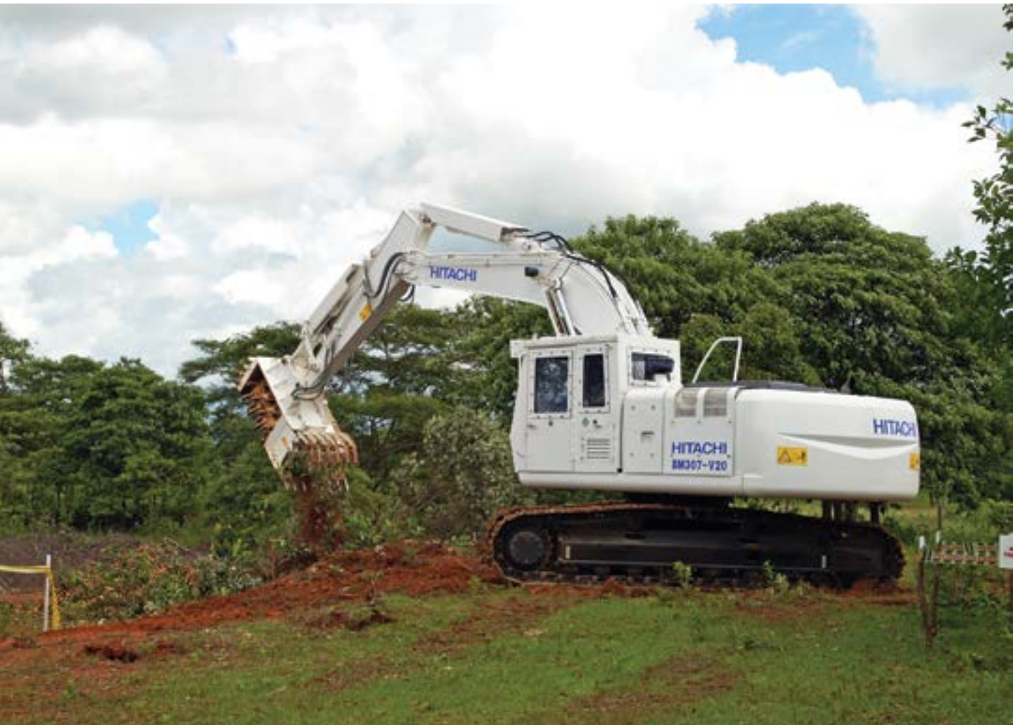
Mechanical demining as part of the land release process. Photo courtesy of the author.
