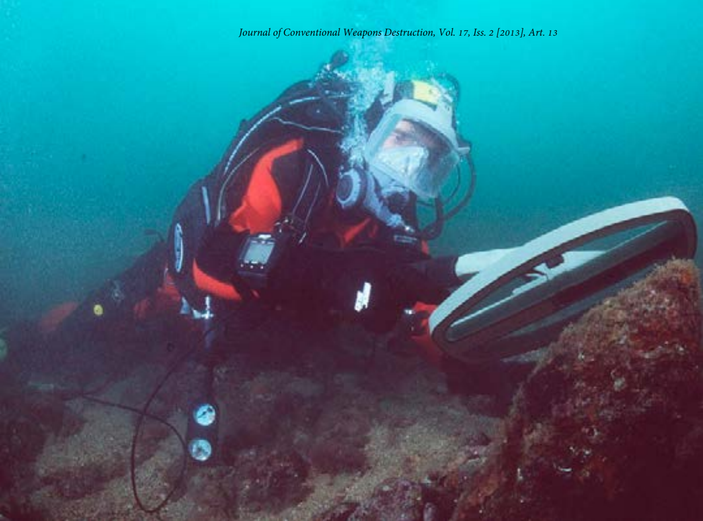
A diver uses an underwater metal detector produced by Vallon to perform underwater mine reconnaissance of the seabed in the Bay of Kotor, Montenegro. All photos courtesy of Regional Center for Divers Training and Underwater Demining.
