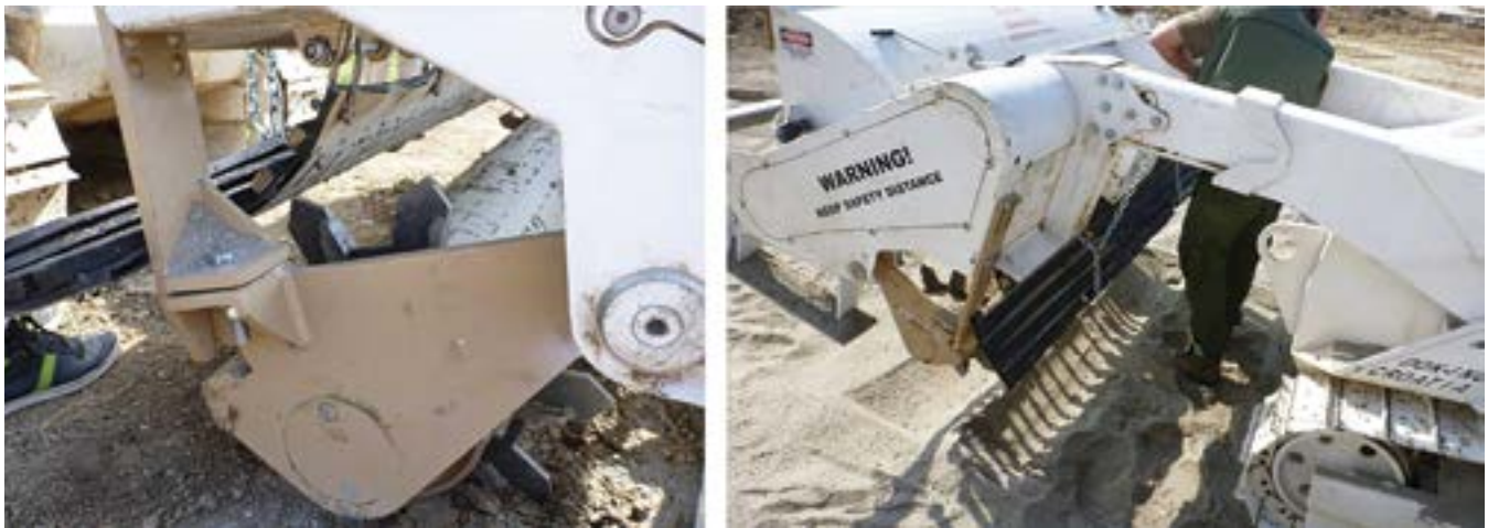
Figure 9. Optimal configuration of the magnetic collection system.
