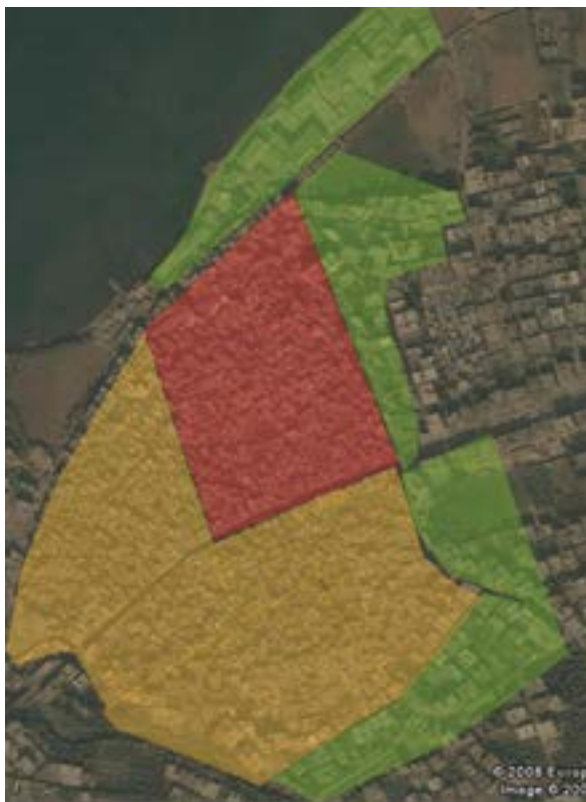
Figure 4. NBC risk assessment by MAG. UXO-contaminated zones: Red area—heavy density (50 to 125 units of UXO per hectare) and possible five unexploded 250 kg air bombs; Amber area—normal density (13-49 units of UXO per hectare); Green area—light density (6-12 units of UXO per hectare). Figure courtesy of MAG, Risk Assessment Report, April 2008.
