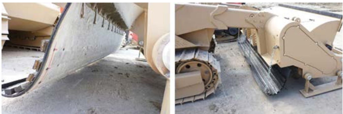
Figure 3. Magnetic sheet attachment.
