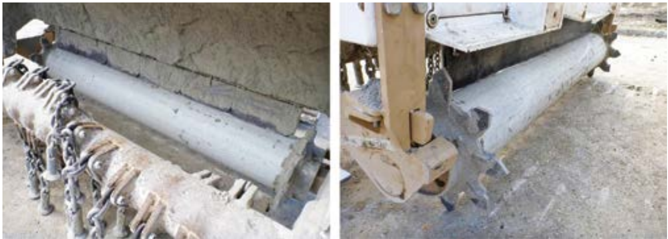
Figure 2. Magnetic roller attachment.
