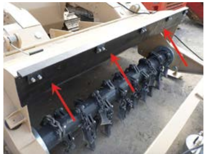
Figure 4. Magnetic upper catch attachment.
