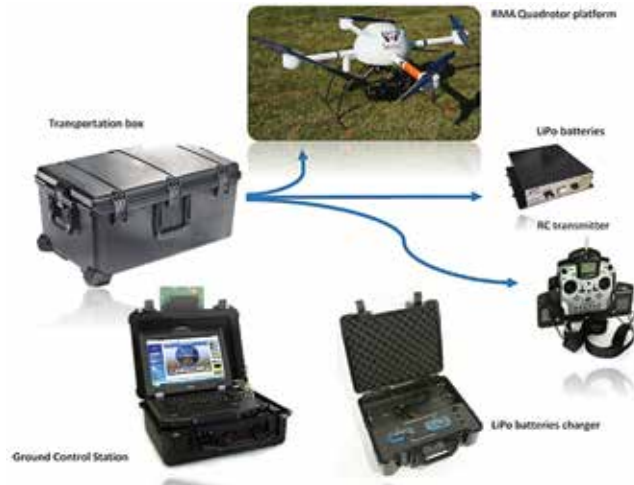
Image 1. RMA's remotely piloted aerial system.
