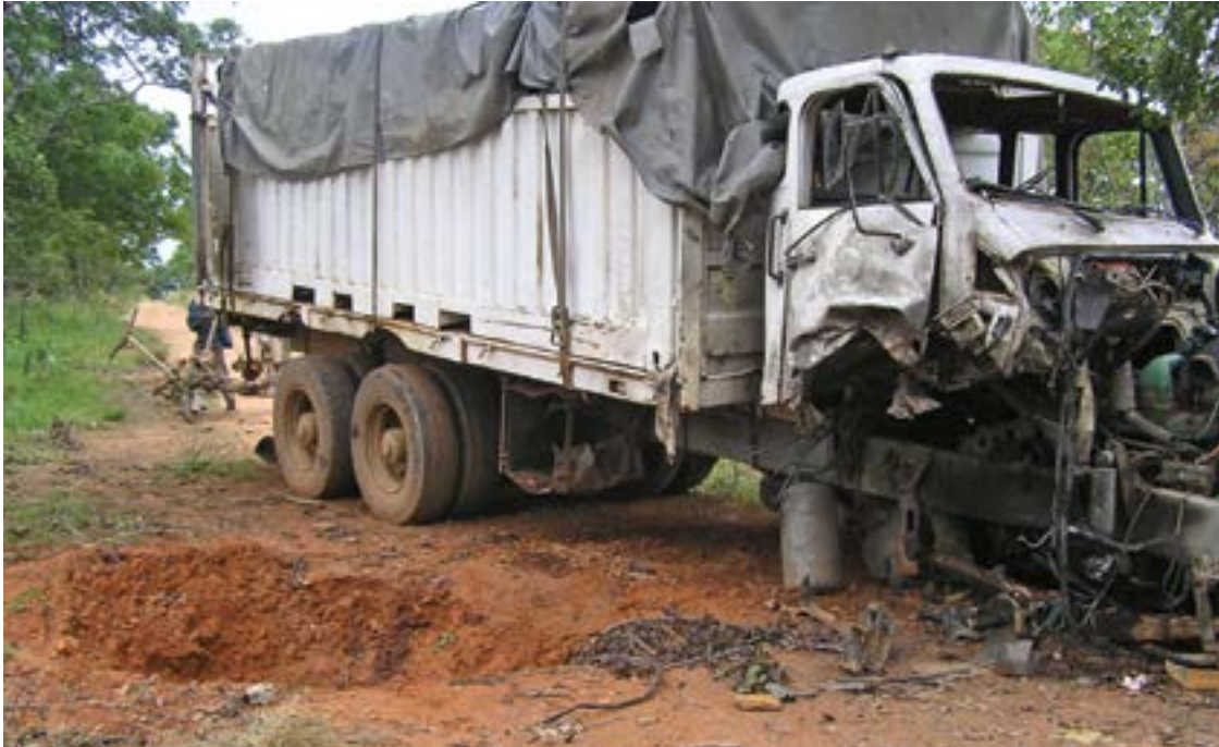
A truck damaged by the blast of an anti-vehicle mine in Angola. Photo courtesy of The HALO Trust.
