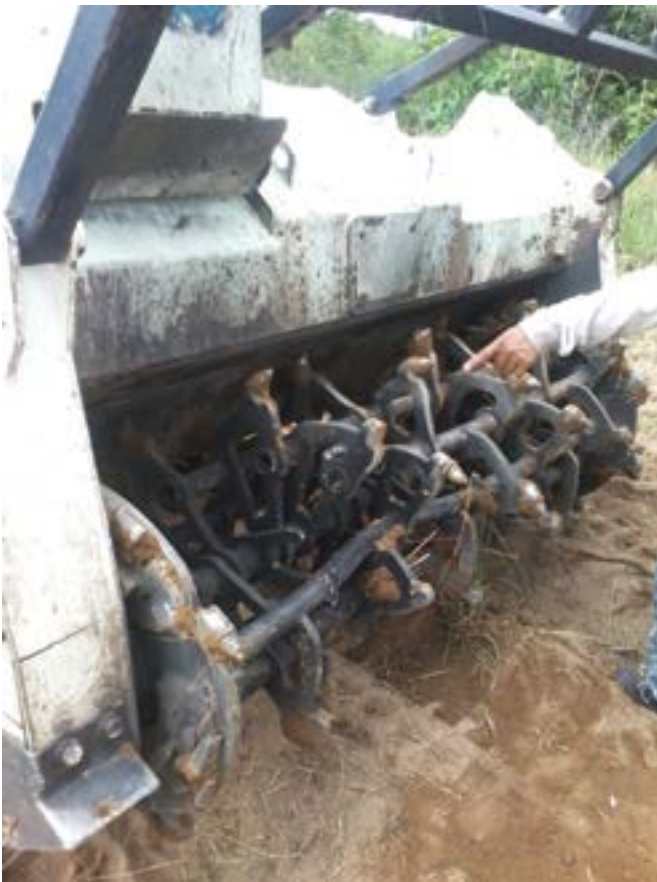
The tiller of the Mini MineWolf is capable of detonating AP mines without sustaining any damage. Photo courtesy of HD R&D.
