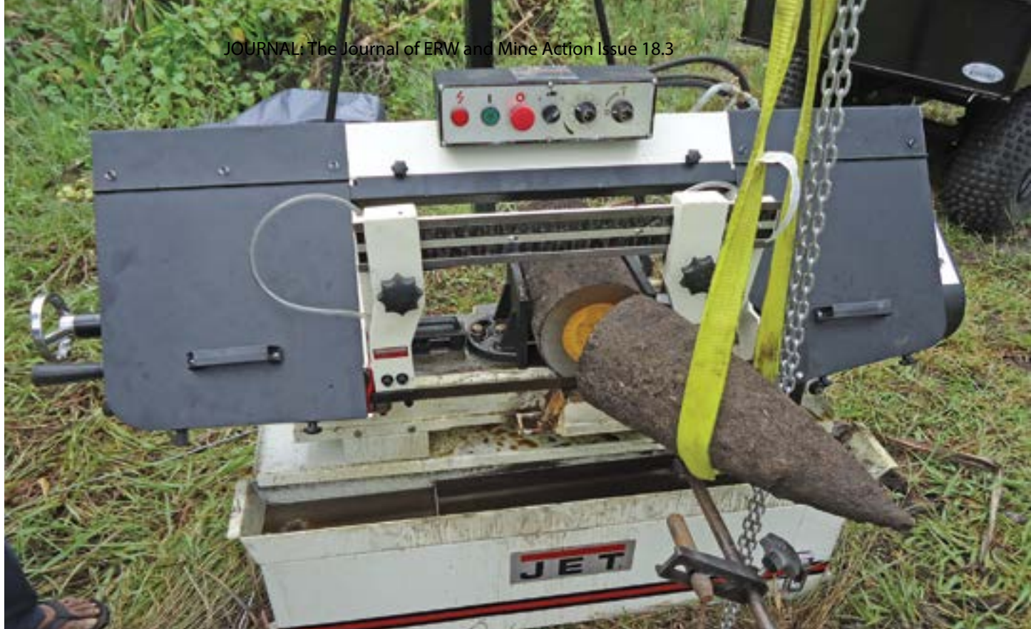
Golden West's Mobile Bomb Cutting System.
