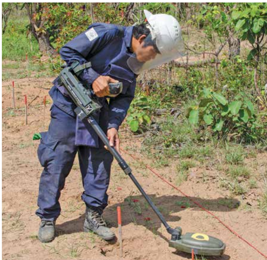
A MINEHOUND VMR2 is used to find AP mines in Cambodia. The use of this system allows 92% of signals from metallic rubbish to be rapidly excavated.
