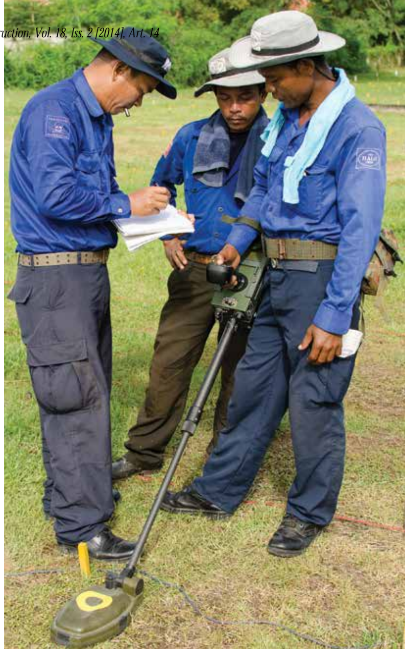
Deminers in Cambodia are taught how to calibrate the GPR on the MINEHOUND VMR3 using buried test targets chosen for the expected threat in the minefield.
