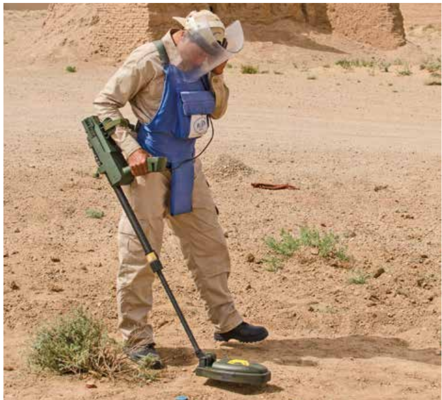
A MINEHOUND VMR3 in an AT minefield in Afghanistan. The large size of the expected mines means that the GPR can be calibrated to ignore nearly all other signals.
