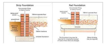
Figure 5 Strip and pad foundation for expansive soil
