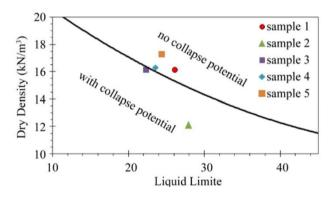
Figure 3 Collapse potential to Liquid Limit and Dry Density
