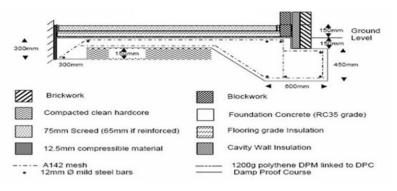
Figure 4 Raft foundation on expansive soil
