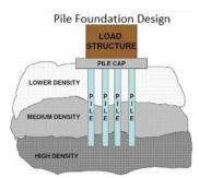
Figure 6 Pile foundation in expansive soils
