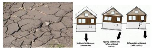
Figure 2 Expansive soil and its effect on buildings
