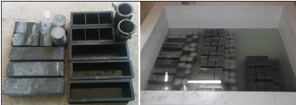
Figure 5 Prism and cube samples
