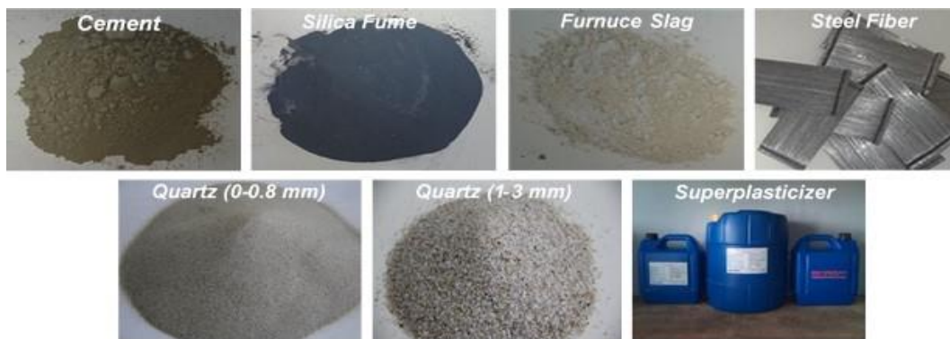
Figure 7 Material components of the UHPFRC
