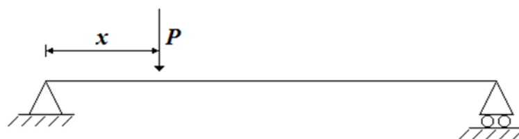
(a) Force at a fixed point, x , on the beam with P=100kN .
