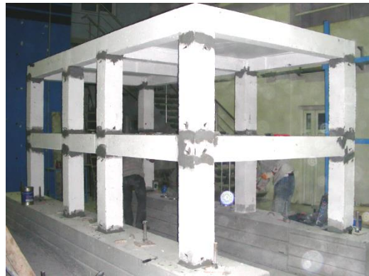
Figure 8 Repaired RC reference model before strengthening
