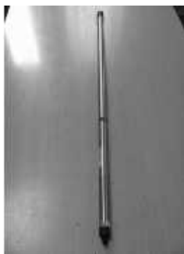
Figure 9 a) e+ WATER L level sensors
