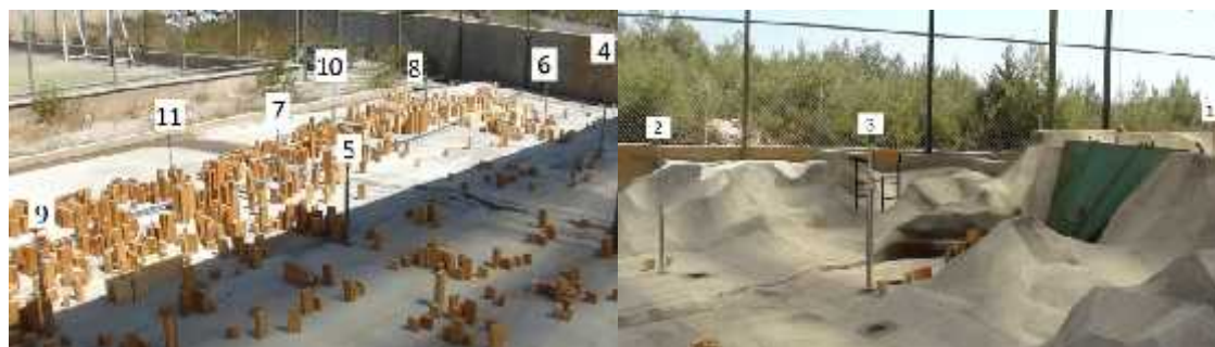
Figure 10 Locations of the level meters and UVP transducers
