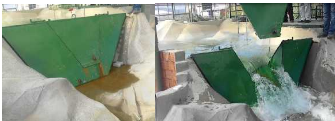
Figure 11 The mechanism of the partial dam break
