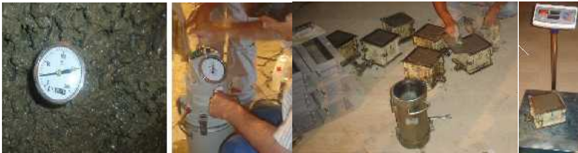
Fig. 1 Measuring the temperature and porosity on concrete
