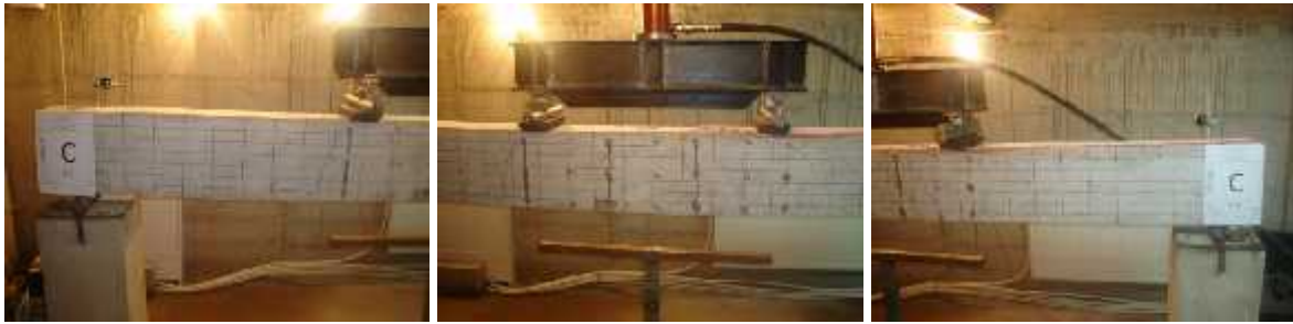
Fig. 4. Testing of beam in failure on the time t = 400 days
