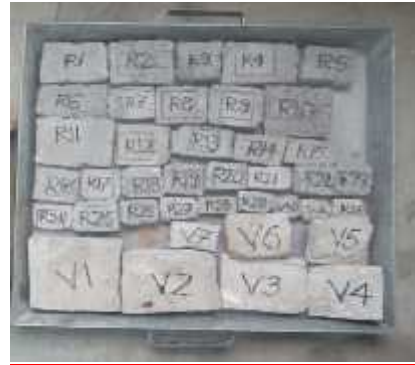
Figure 4 Mortar samples cut into regular forms
