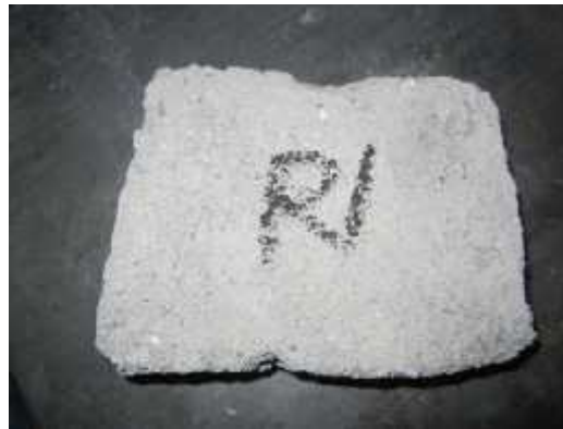
Figure 6 Cut mortar specimen
