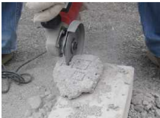
Figure 5 Mortar specimen being cut
