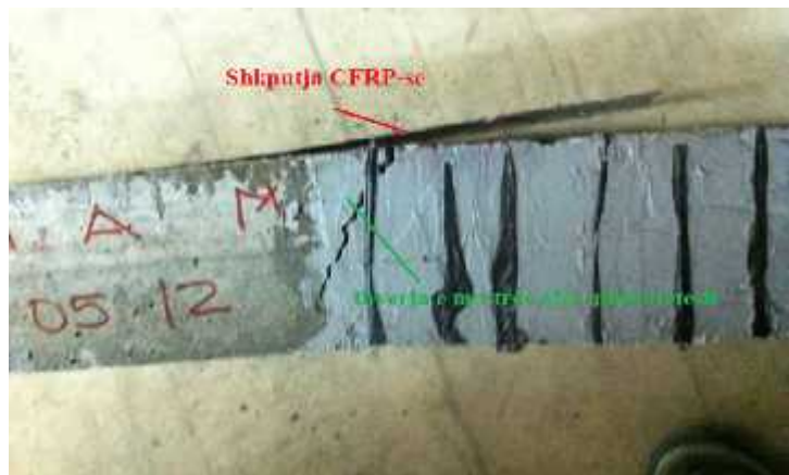
Fig.5.2-delaminate of the CFRP in Set A/beam 3
