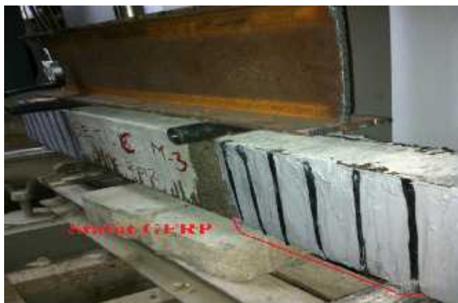
Fig.5.6 Cracks in Set C/beam 3
