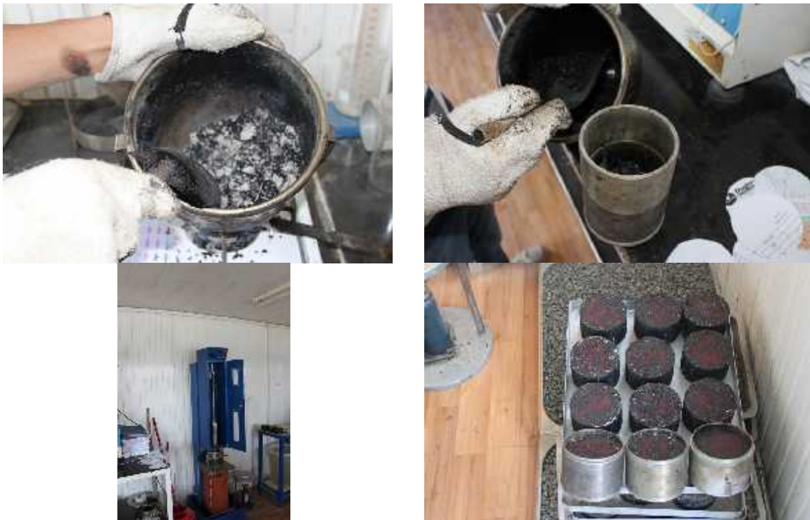
Figure 2 Marshall sample fabrication process
