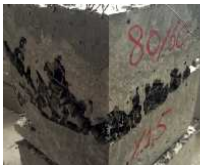
Figure 4 A cube specimen produced with 80/60 fiber type and 1.5% fiber volume fractions contains spaces
