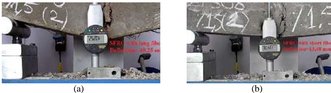
Figure 6 At the end of bending tests, deflection of SFRC specimens with long (a) fibers and short (b) fibers
