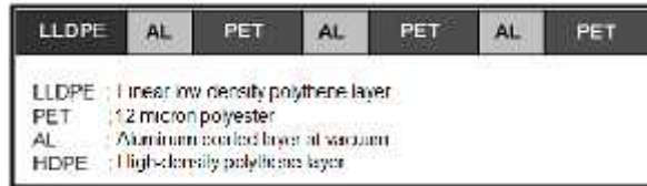
Figure 7. An example outer barrier (metalized film) layers used in VIP production.
