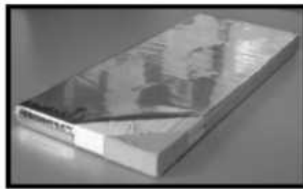
Figure 5. View of a core, inner and outer envelopes of a VIP.
