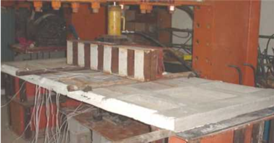
Figure 1: set-up of test for two line load test
