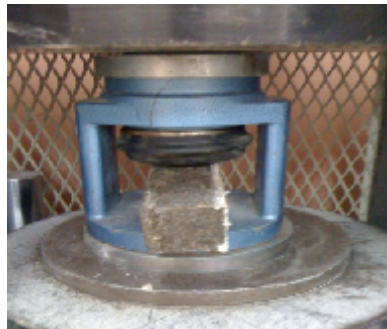
Figure 4. Compression Strength Test
