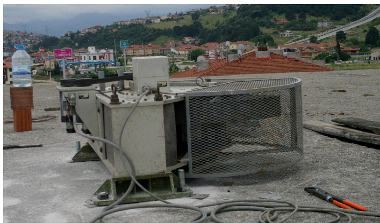
Figure 2 Vibration generator manufactured by Kinematics mounted at the top of the building
