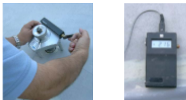
Fig.9. a/ examinations of bonding strength; b/ the results of bonding strength
