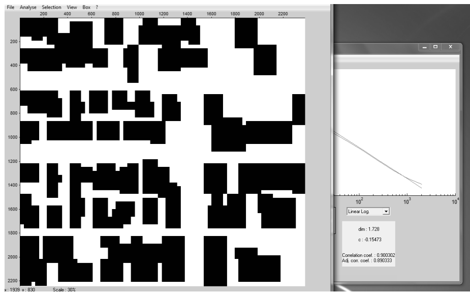
Figure 3: Measuring the fractal dimension of the Korca's vernacular pattern using Fractalyse as software. Fractal dimension value 1.728; Scale 2
