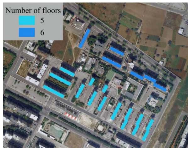
Figure 5: Thematic map of buildings of studied area, according to the number of floors
