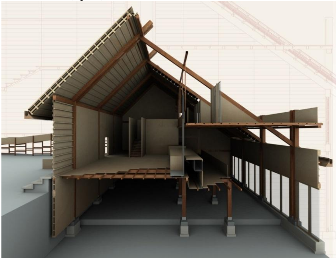
Figure 4: Perspective cross section showing the wooden supporting structure of the museum (V.Dario)
