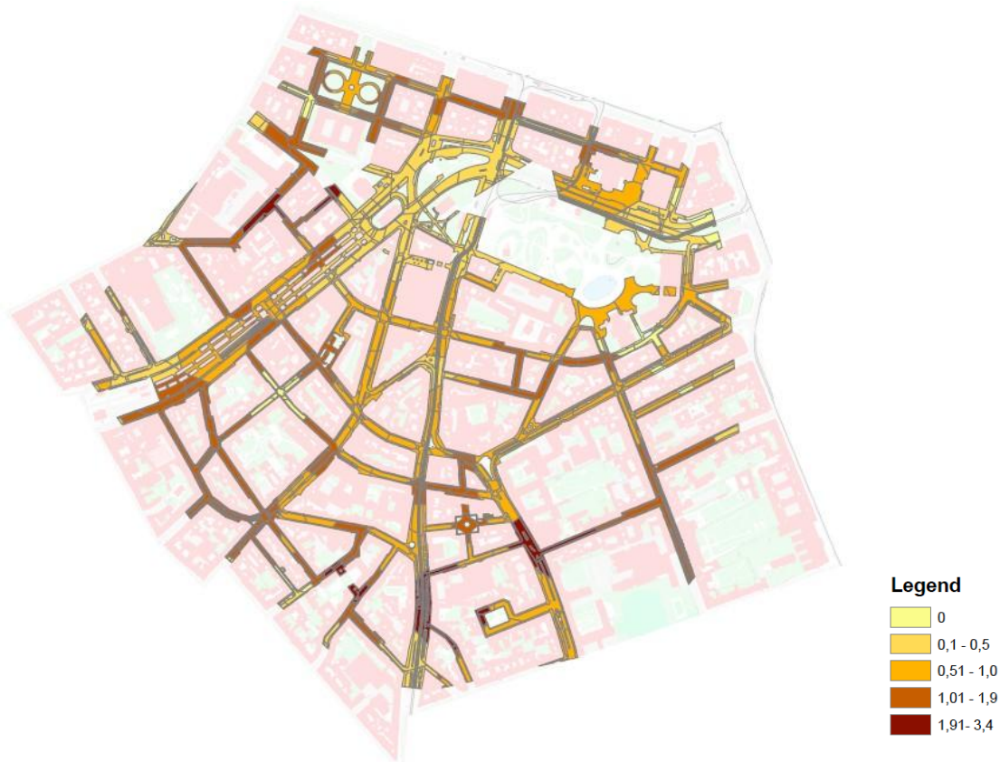
Figure 5: Automated aspect ratio calculation for the city center of Vienna.
