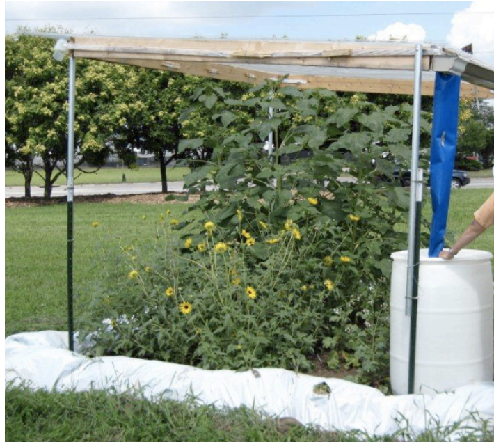
Fig. 2. Rain-out shelters used to capture rainfall. Rainfall hit the transparent roofing, was caught in the rain gutter, and drained into a rain barrel. The rain was then redistributed using a 4-hp water pump and tractor.
