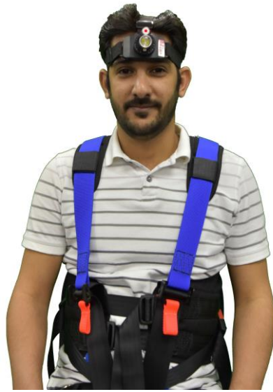
Figure 3. Participant was fitted with a safety harness and performed horizontal and vertical head motions using a head-mounted laser pointer to guide amplitude.
