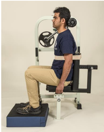
Fig. 5. Subjects in experimental group sat with their head and neck in neutral position. To limit the involvement of trunk muscles during the 5-minute isometric exercise, a regular gait belt was used to harness the trunk to the back support.
