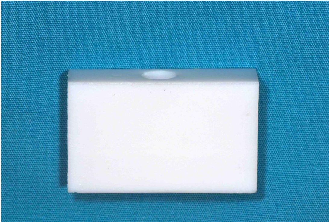
Figure 2. Teflon mold used to fabricate the composite resin grips
