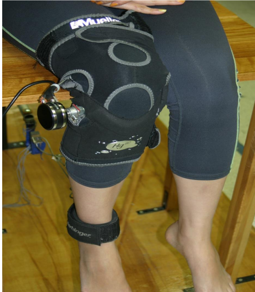
Figure2. Experimental setup for measuring FFK and FEK of the knee, the subject was positioned sit with their hip and knee flexed to 90 degrees.
