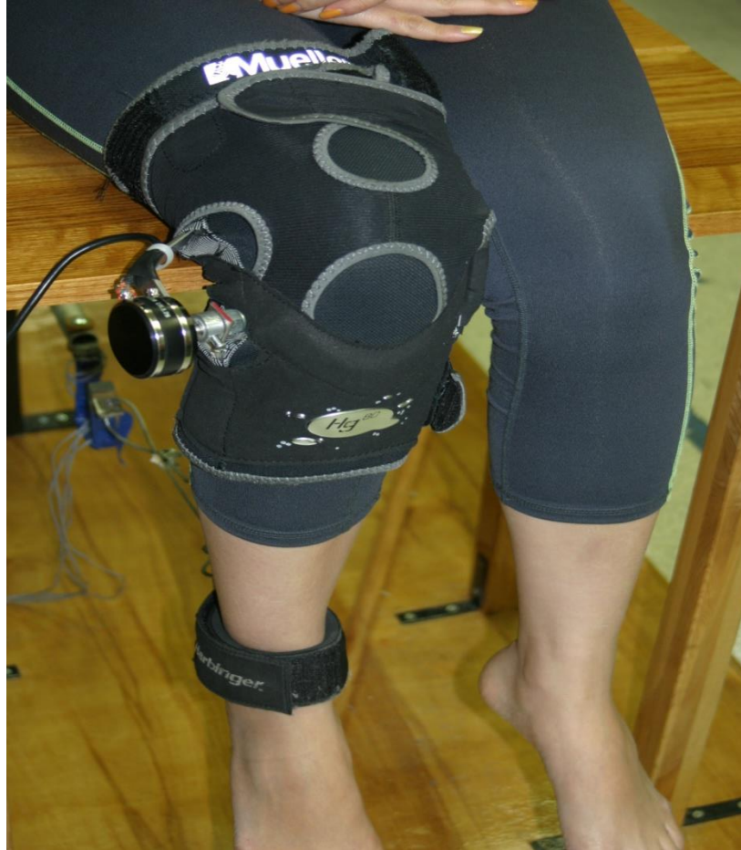
Figure9. Experimental setup for measuring FFK and FEK of the knee, the subject was positioned sitting with their hip and knee flexed to 90 degrees.
