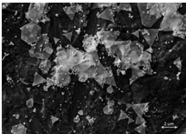
Figure 3.8 (A) STEM image with initial 10^{-3} M Au(III) concentration after 3 days for L31:F68/(8 mM: 4 mM) aqueous solution. (B) FESEM image of Au nanoprisms with initial 10^{-3} M Au(III) concentration reduced in a L31:F68/(8 mM: 4 mM) aqueous solution.
