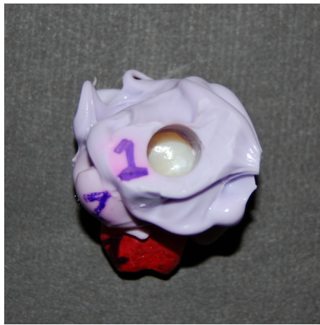
Figure 2: Custom jig fabricated for each tooth specimen to increase the precision and repeatability of L* measurements
